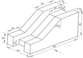
Draw its i) Front view ii) Top view and iii) side view of the object shown in figure. All Dimensions are in mm
